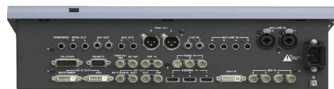
A rear view of the Sony MCS-8M, for a close look at the various HD and SD inputs and DVI outputs that the video switcher provides.
