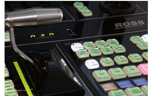
Among the aspects to consider that are part of a switcher, as shown to the right in this image with this Ross switcher, are the number of keyers that are included.
