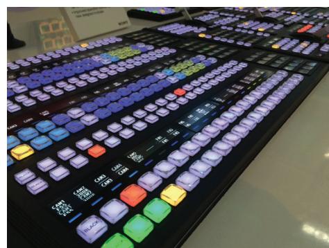
The Sony XVS-8000, the flagship video switcher produced by the Japanese manufacturer.
